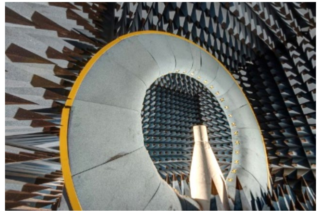
Figure 7: Anechoic chamber for testing total efficiency - full 3D pattern is measured.
