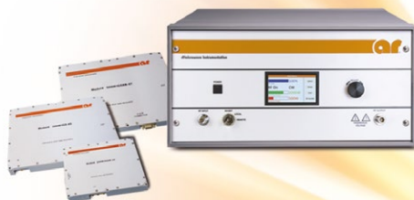
Solid State 700 MHz to 6 GHz, Single Band Amplifiers, Hybrid Modules to 50 Watts, Benchtops to 500 Watts CW Class A designs for linear applications; Class AB designs for increased power and efficiency. Applications include EW, reliability stress screening and EMC test.
