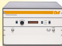
Solid State 700 MHz to 18 GHz Dual Band Amplifiers AR offers the widest Class A solid state frequency range coverage in a single amplifier housing. These amplifiers come in a split band configuration from 0.7 to 6.0 GHz up to 60 watts and 6 to 18 GHz up to 40 watts CW. It costs less, weighs less, and takes up less space than two separate amplifiers.
